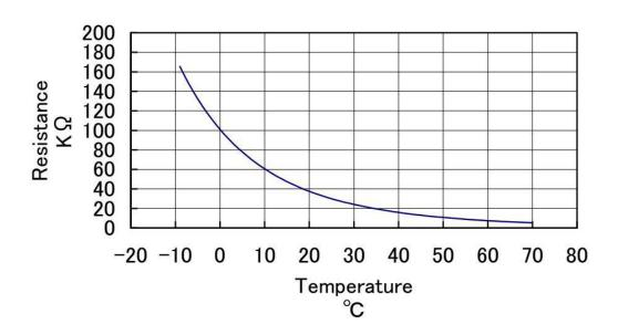
$R_X = R_{25} * EXP\{B*(1/T_X-1/T_{25})\}$ (T; Absolute temperature)
