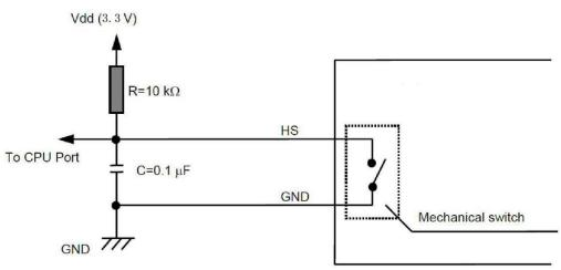
\* The mechanical switch is opened when the lever is in an OPENED state.
