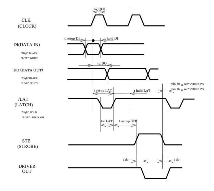
\*If delay time for Driver Out can not be secured enough, there is a possibility that VH would fluctuate greatly. Please design the circuit so that VH does not exceed peak voltage (Vp).
